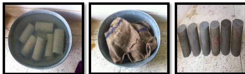
Fig. 3. Curing and drying of concrete cylinder
